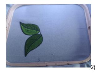
Stitch color 3, the placement indicator for the piece of HTV. Cut it a little bigger than the color just stitched and remove the sticky plastic foil.
